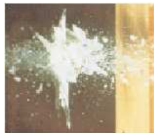
Bullet-resistant acrylic The same bullet also explodes through 1-1/4" thick bullet-resistant acrylic, scattering a shower of fragments.
