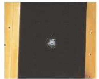
LEXGARD SP 1250 laminate 1-1/4" thick LEXGARD SP 1250 laminate can absorb full ballistic impact without penetration or shattering.
