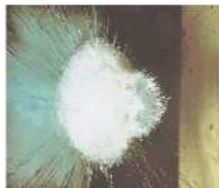
Bullet-resistant glass A .44 Magnum bullet shatters 1-3/16" thick bullet-resistant glass, creating a dangerous situation.
